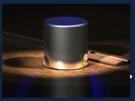
The unit of mass the kilogram, was defined until May 20, 2019 as the mass of a chunk of platinum in Paris, shown here.
