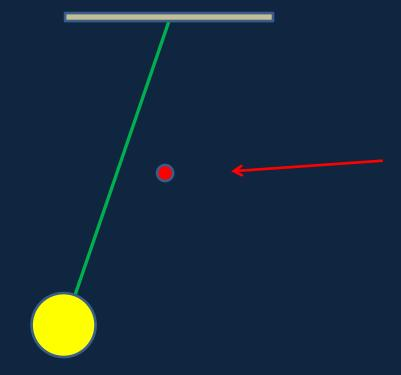
First he took a pendulum swinging freely back and forth, then he introduced a fixed peg directly below the point the pendulum hangs from.
