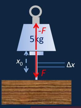
Weight hits nail with speed  $v_0$
