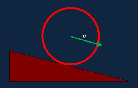
The hoop takes longer to get down than a low-friction sliding block, because the same loss in potential energy has to supply BOTH translational *KE* and rotational *KE* for the hoop.
