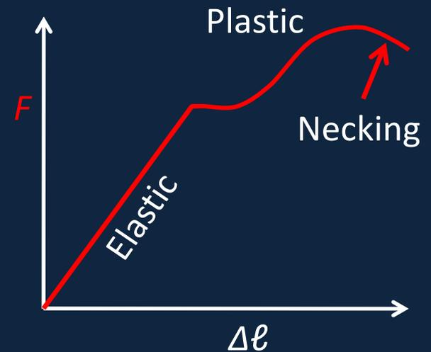
The shape of the curve in the plastic region differs from one substance to another—just before breaking, narrowing often occurs at one place : “necking”.
