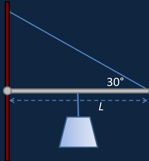
The distance from the hinge to the line of action of the force is  $L\sin 30 = L/2$ .
