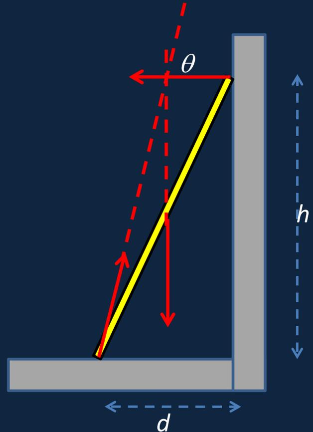
**Warning:** this trick saves working with components, but does NOT work if there are more than three forces! (Someone on the ladder.)
