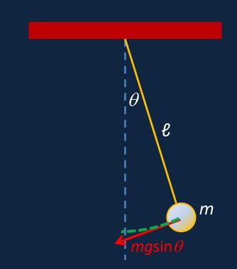
The time for a complete swing doesn't depend on the mass *m*, for the same reason that different masses fall at the same rate.
