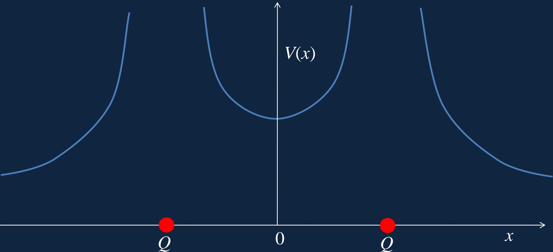
Note: the origin (at the midpoint) is a “**saddle point**” in a 2D graph of the potential: a high pass between two hills. It slopes **downwards** on going away from the origin in the  $y$  or  $z$  directions.
