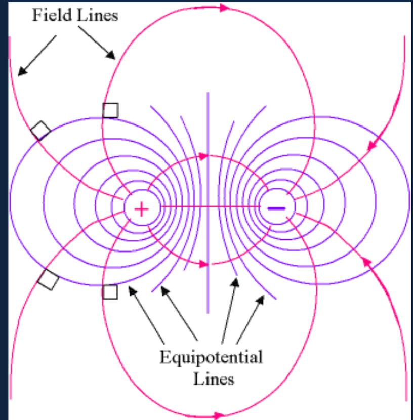
Here's a more physical representation of the electric potential as a function of position described by the equipotentials on the right.
