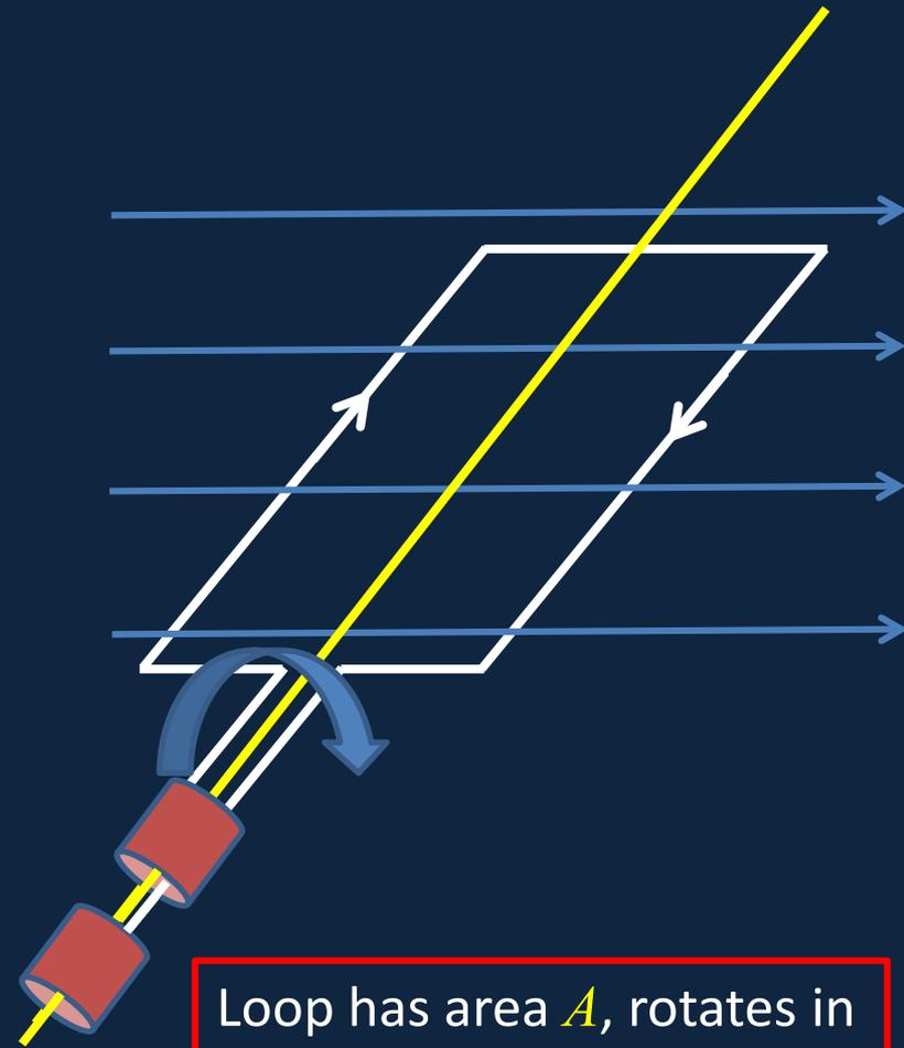
Loop has area  $A$ , rotates in field  $B$  at  $\omega$  radians/sec.
