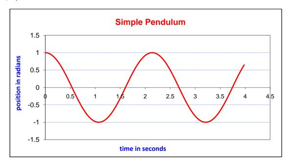
The change in period is a little less that 10%, not too dramatic considering the large amplitude of this swing. Two radians gives an increase around 35%, and three radians amplitude increases the period almost threefold. It's well worth exploring further with the <a href="mailto:spreadsheet">spreadsheet</a>!
