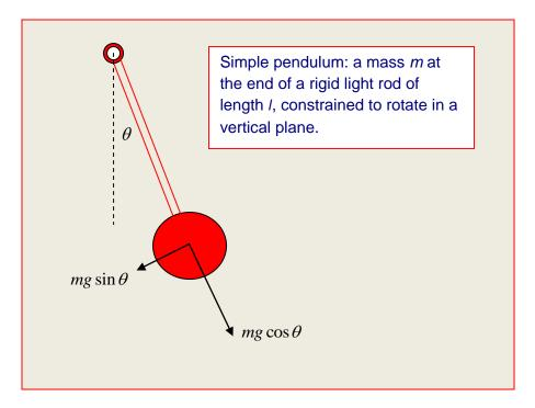
In fact, though, the pendulum is not quite a simple harmonic oscillator: the period *does* depend on the amplitude, but provided the angular amplitude is kept small, this is a small effect.
