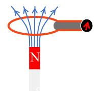
response current builds up in the ring, it generates a repulsive force so it takes work to keep moving the magnet, this is the source of the energy needed to build up the current in the ring (which then dissipates as ohmic heat).
