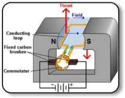
One common electric motor design is just the "loop in a magnetic field" generator we already discussed, but now run backwards—by which we mean power is supplied from a battery, say, to the loop which then becomes a dipole-like electromagnet. The loop is between the poles of a permanent magnet so it turns, but as it reaches the limit a commutator reverses its current supply, so attraction suddenly becomes repulsion and since it's rotating it continues around, whereupon the sequence repeats.
