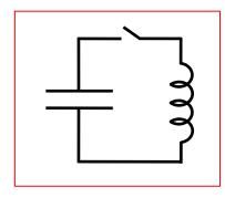
We first assume there's zero resistance, just *C* and *L* in series, with an open switch. We charge *C*, then close the switch. Charge will begin to flow through the inductance from one plate of *C* to the other. The current I = -dQ/dt will build up, but its **rate of increase will depend on the inductance**, the back emf LdI/dt balancing the voltage Q/C of the capacitor.
