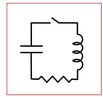
This equation for Q is **identical** to the equation of motion for x for a **damped** mass on a spring: imagine a mass in molasses. L is the mass, 1/C is the spring constant k and R is the damping term b: see that earlier work.
