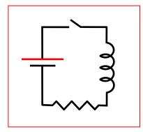
A battery is connected to *L*, *R* in series:  $V_0 = IR + L\frac{dI}{dt}$ .
