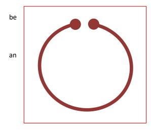
It's also worth mentioning here that this *L*, *C* circuit can very simple: for example, a ring with a gap:
