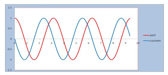
Current and emf in a purely capacitative AC circuit: current leads emf by a quarter cycle (ICE).
