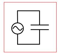
Putting  $V=V_0\cos\omega t$  across a capacitor, again with no resistance (or inductance) in the circuit, at t=0 the voltage is at its maximum positive value, which means the capacitance contains its maximum positive charge in the cycle. At that moment, the current must be zero: the capacitance has charged up fully, and is about to begin discharging as it follows the cycle.
