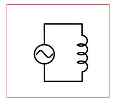
If we put an alternating voltage across an **inductor** *L*, having zero resistance *R*, this external voltage must be exactly matched by the back emf generated.
