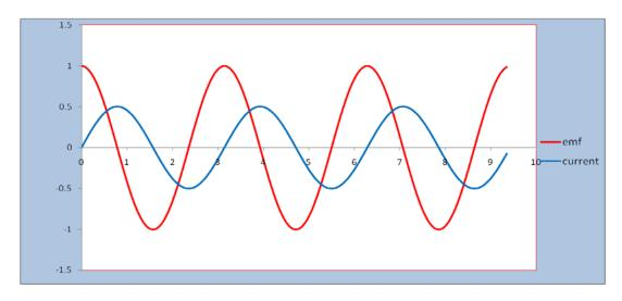
Current and emf in a purely inductive AC circuit: emf leads current by a quarter cycle (ELI).
