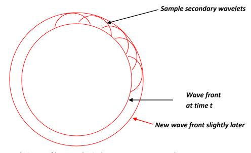
Huygens' picture of how a spherical wave propagates: each point on the wave front is a source of secondary wavelets that generate the new wave front.
