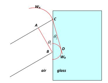
Huygens' explanation of refraction: showing two wavelets from the wavefront AB.  $W_B$  is slowed down compared with  $W_A$ , since it is propagating in glass. This turns the wave front through an angle.
