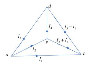
An Example: Compute the resistance  $R_{ac}$  of this network from a to c given that all lines are one ohm resistors except dc, which has resistance r.
