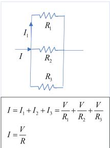
Parallel resistances all have the same voltage drop, the total resistance (see figure) is given by
