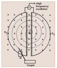
The two "D"s are hollow D-shaped metal boxes, open along the straight part.
