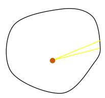
Suppose now we take a *noncircular* contour for the integral. The increment  $\vec{B} \cdot d\vec{\ell}$  only has a contribution from the component of  $d\vec{\ell}$  which is parallel to  $\vec{B}$ , and has length  $rd\theta$ , so we get the same result for the integral.
