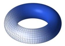
A toroid here is equivalent to a solenoid with the axis turned into a circle so the two ends connect. This is a promising design for containing a hot plasma, unlike the "magnetic bottle" where charged particles can escape at the ends.
