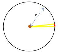
Consider a current I in a long wire perpendicular to the screen, and the integral  $\oint \vec{B} \cdot d\vec{\ell}$  around a circle of radius r as shown. Taking  $B = \mu_0 / 2\pi r$ , and  $d\ell = rd\theta$  (the small red vector), the integral is just over  $\theta$  from zero to  $2\pi$  and
