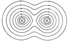
The field from current  $I_1$  is  $B = \frac{\mu_0}{2\pi} \frac{I_1}{r}$ , circling the wire, and the current  $I_2$  will feel a force  $I_2 \vec{\ell} \times \vec{B}$  per length  $\ell$ , so the force per meter on wire 2 is
