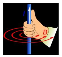
From many experiments, the lines of magnetic force are circles around the wire, direction determined by the right-hand rule.
