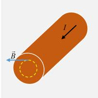
Apply Ampère's law to the dashed circular path of radius r inside the wire as shown. From symmetry (and no monopoles), the field must be tangential.
