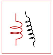
More generally, if two coils 1, 2 are in proximity, a current through one will cause some magnetic flux to thread through the other, so a changing current in one will induce an emf in the other. From the Biot-Savart Law, the magnetic field from a current is linear in the current (directly proportional to it) so from Faraday's law, the induced emf will be linear in the rate of change of the current  $I_1$  in coil 1.
