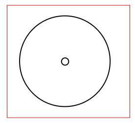
Another example: consider a small circular loop at the center of a large circular loop, both in the same plane. Putting a current I in the big loop gives a field on the axis at the center of  $\mu_0 I/2R$ , so if the small loop has r << R, we have
