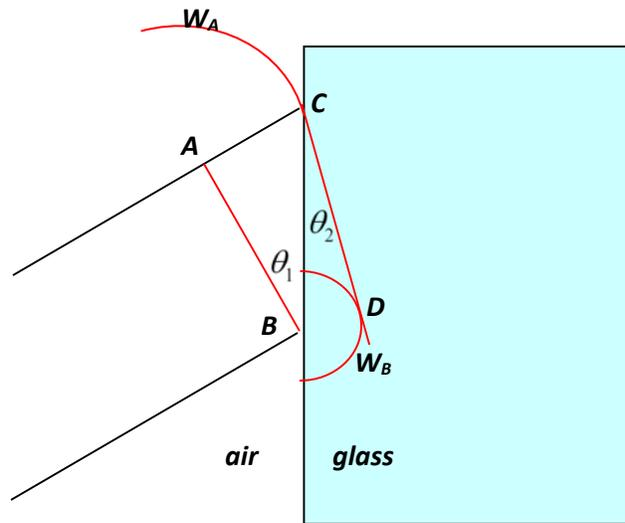
***Huygens' explanation of refraction: showing two wavelets from the wavefront AB.  $W_B$  is slowed down compared with  $W_A$ , since it is propagating in glass. This turns the wave front through an angle.***
