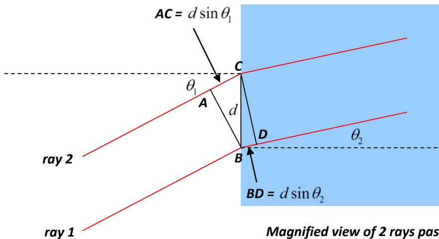
**Magnified view of 2 rays passing through interface: ray 1 is the minimum time path. Rays encounter interface distance  $CB = d$  apart.**
