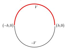
circle is in segments at different potentials. The simplest case has the top and bottom halves of a circular pipe at different potentials, say  $\pm V$ .
