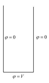
Suppose a duct is open on one side, or rather that the two neighboring sides go to infinity in our approximation, and these sides are kept at zero potential. The bottom side in the diagram is kept at constant potential  $\varphi = V$ .
