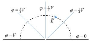
Infinite conducting sheet in (x, y) plane, thin gap along y axis. Sheet x < 0 at potential V, sheet x > 0 grounded.
